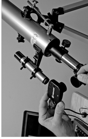
Fig. 11: Insert the PC Camera into the telescope's eyepiece holder.
